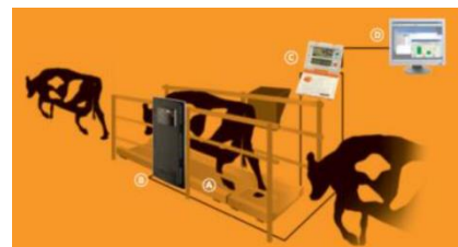
Photo 5. Walkover weigh scale system. Source: WUR
