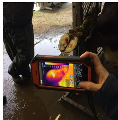
Photo 9: Lesion detection in a claw by using a handheld thermal imaging camera (Miracle Tech)
