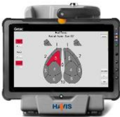
Photo 7: Rubber mounted tablet with software to record hoof problems and treatments (Supervisor System™)
